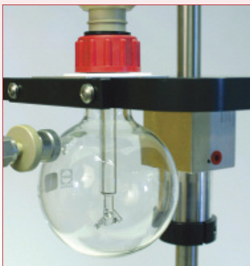
Leak-tight stirrer assembly
